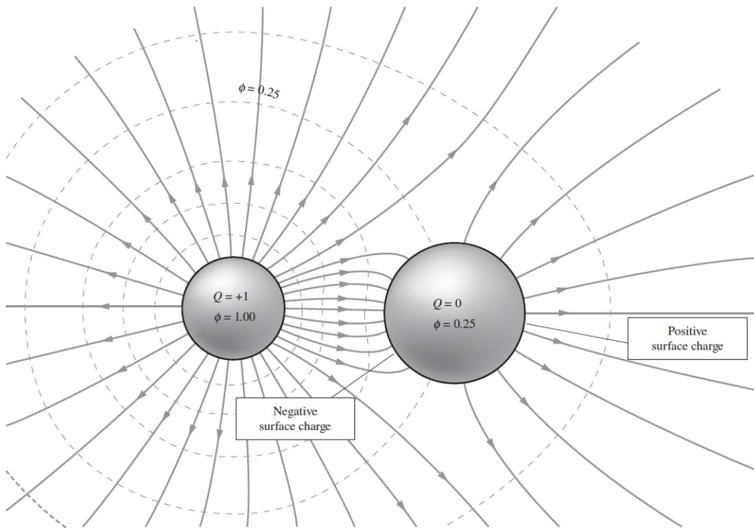
Notice how the field lines are normal to the equipotential lines. The neutral sphere has zero net charge but non-zero electric potential. This means it would take work to bring a test charge from infinity to the surface of the neutral sphere.
